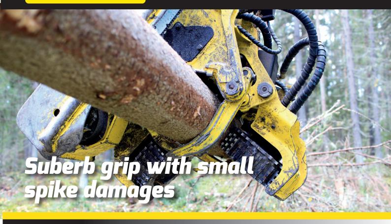
Moipu Flex standard feed rollers are known for their large gripping surface, which results in immense feeding force.
